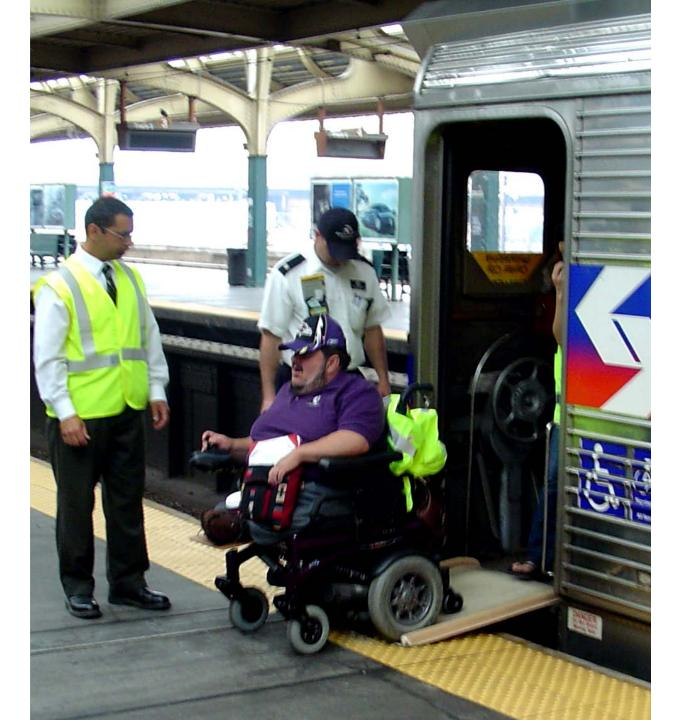
Exiting at grade from older rail car at historic station, using movable bridgeplate.
